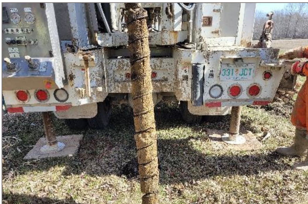
Photo 13: General view of the brown silty sand layer found on the site. (May 11, 2021)
